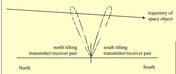
Ensured correlation of same object establishes single pass orbit determination
