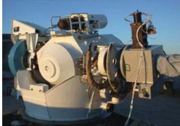
For the first time in Russia, a 28-channel adaptive optical system has provided spacecraft images.
