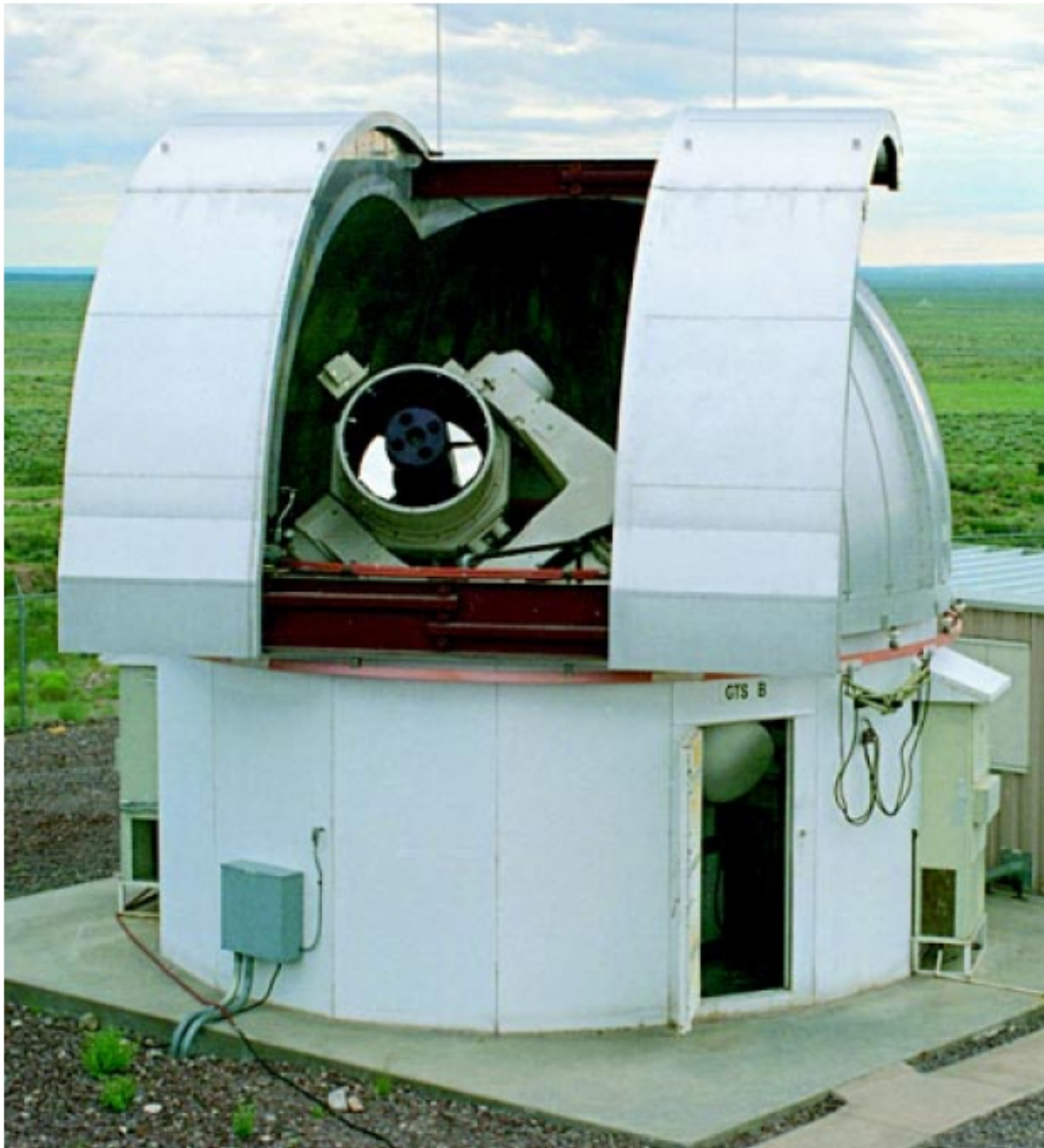
One of two one-meter Ground-Based Electro-Optical Deep-Space Surveillance (GEODSS) search telescopes at the Lincoln Laboratory Experimental Test System (ETS) at White Sands Missile Range, New Mexico. This telescope, which previously was used for space surveillance, is now a component of the Lincoln Near-Earth Asteroid Research (LINEAR) asteroid search program.
