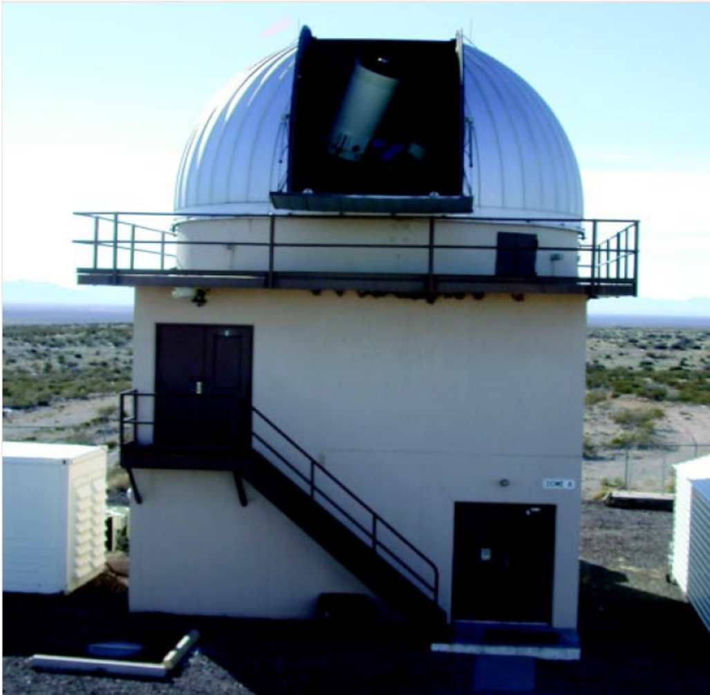
FIGURE B. The LINEAR 3 telescope and its dome at the Lincoln Laboratory–operated Experimental Test System in New Mexico. It is a Cassegrain telescope with a thirty-inch aperture and a 0.5 square-degree field of view. It can routinely detect objects with a visual magnitude of 19.0 with forty seconds of integration. (Photographs courtesy of Peter Trujillo.)
