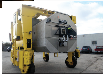
FIGURE 6. The protruding X-band feed is clearly visible in the preupgrade LRIR RF box sitting in the special transporter (above top). An octagonal extension was added to the RF box to house the W-band radar feed, duplexer, and receiver, and radio-astronomy instrumentation—K-band, Q-band, and, in the future, W-band radiometers (right). The HUSIR RF box is shown in the transporter (above bottom).
