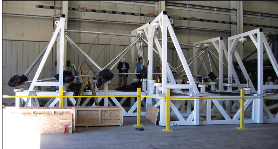
FIGURE 9. The special jigs that Ranor Corporation devised were used to weld nodes (above) and ribs in assembly fixtures (right).
