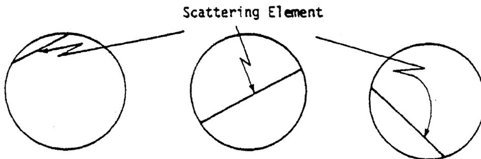
Figure 7. Angular Intensity Measurements Depend on the Location and Orientation of the Dominant Scattering Sources as Well as on Beam Uniformity.
