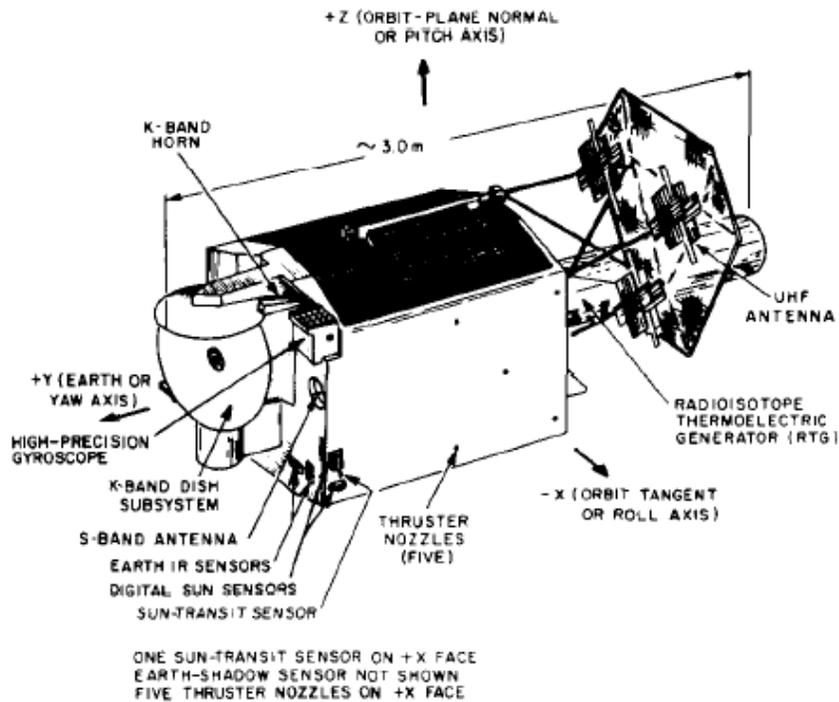
**Fig. 1 Lincoln Experimental Satellites (LES) 8 and 9**
