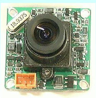
The original 5 inch refractor has been replaced by two CCD cameras each using the well known 1004x sold by RfConcepts in the UK.
