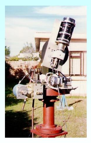
The mounting is able to move in the horizontal (azimuth) as well as vertical plane (elevation) ,each axis being driven by a stepper motor under the control of the program CoSaTrak . The azimuth stepper motor is the blue unit on the left.
