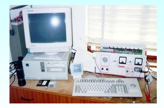
The DOS computer running CoSaTrak and the stepper motors power supply is shown. NOT shown are the video monitors, time unit etc which came later.
